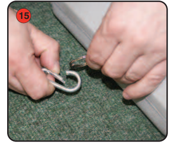
Attach the base springs to each base tank ring.
