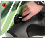
Place the thumbscrew through the graphic holder and tighten until fully secure.
